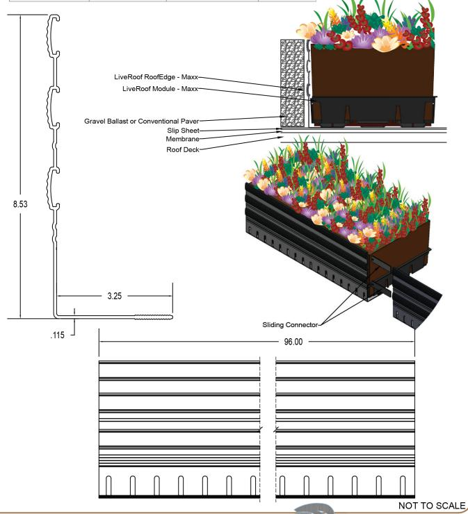
ILLUSTRATIONS ARE TO CONCEPTUALLY ASSIST PROFESSIONALS IN DESIGNING LIVEROOF INSTALLATIONS. LIVEROOF DOES NOT ACCEPT RESPONSIBILTY FOR ENGINEERING BASED ON ILLUSTRATIONS. A QUALIFIED ROOFING SPECIALIST SHOULD BE CONSULTED TO DETERMINE APPROPRIATE WATERPROOFING AND ROOF DECK MATERIALS AND SUITABLE DESIGN.
